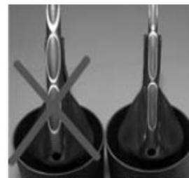
**Do not weld the flooring using the Leister robot without the proper tip.**
